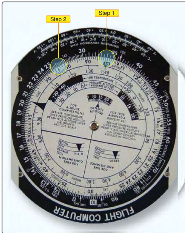
Figure 10-3. E6-B computer set up to multiply 340 by 78.
