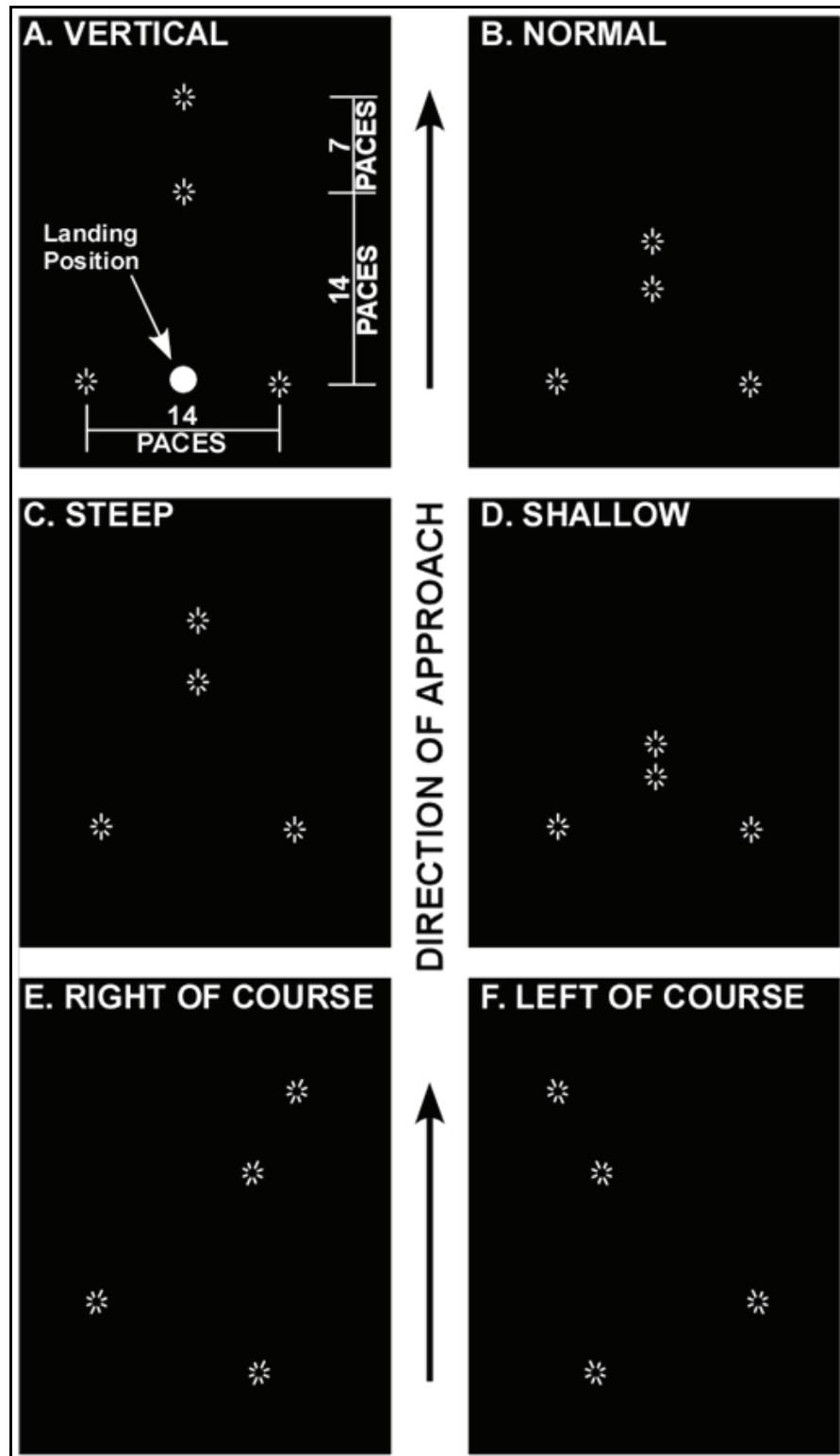
Figure 4-15. Approach to a lighted inverted Y
