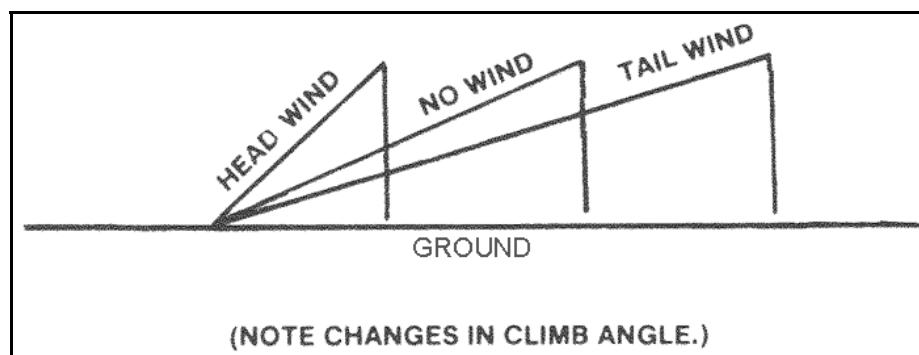
**Figure 7-39. Wind effect on maximum climb angle**
