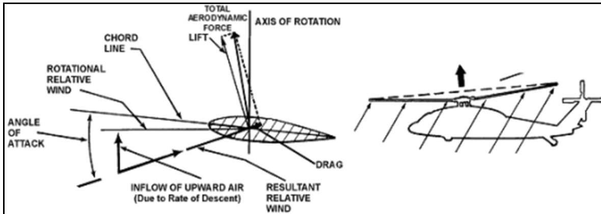
**Figure 1-66. Force vectors in autorotative steady-state descent**
