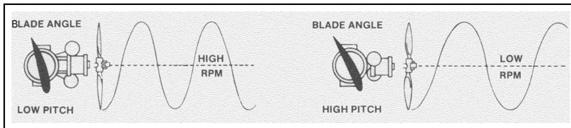
**Figure 7-58. Blade angle affected by revolutions per minute**
