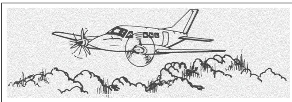
**Figure 7-62. Windmilling propeller creating drag**
