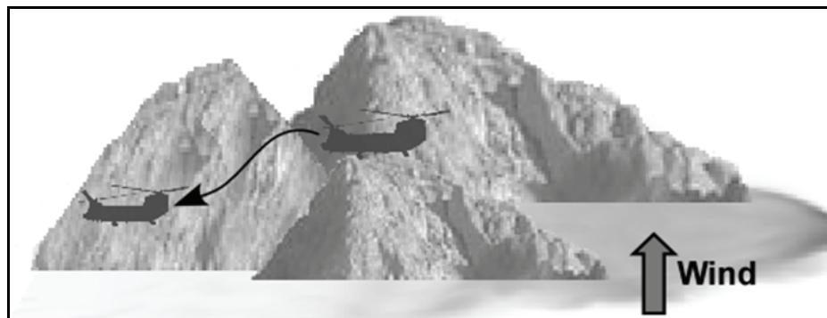
**Figure 3-26. Nap-of-the-earth or contour takeoff (terrain flight)**
