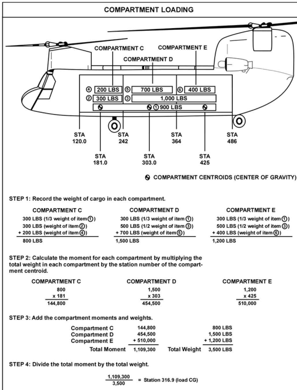
**Figure 2-11. Compartment method steps****Station Method**
