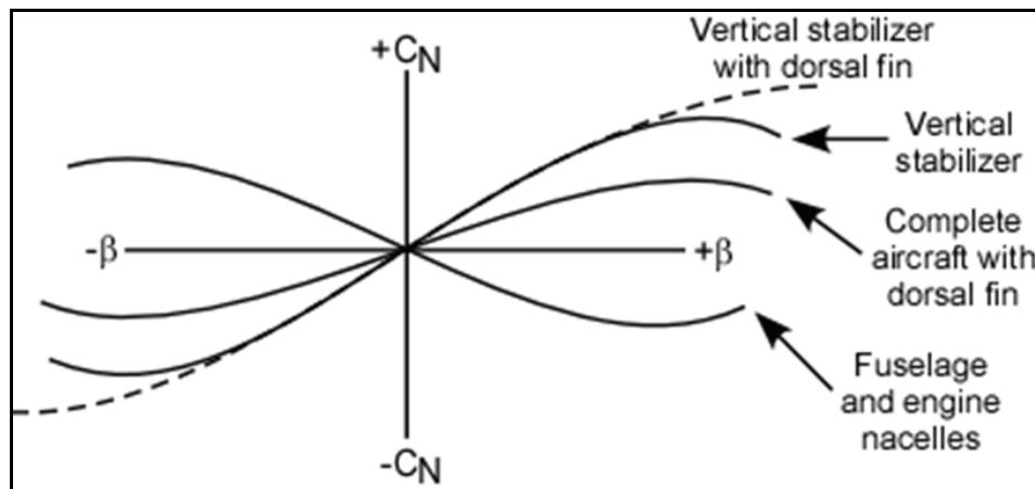
Figure 7-15. Fixed-wing aircraft configuration positive yawing moment
