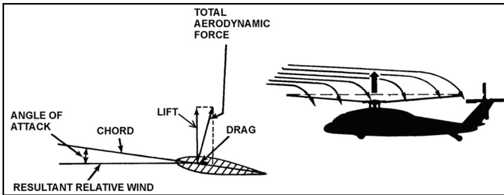
**Figure 1-65. Force vectors after power loss-reduced collective**
