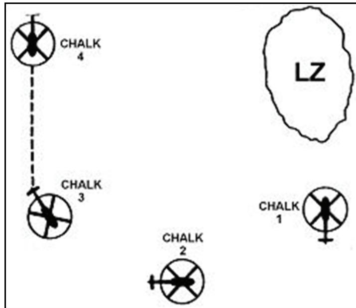
**Figure 6-4. Left break with 10-second interval for landing**
