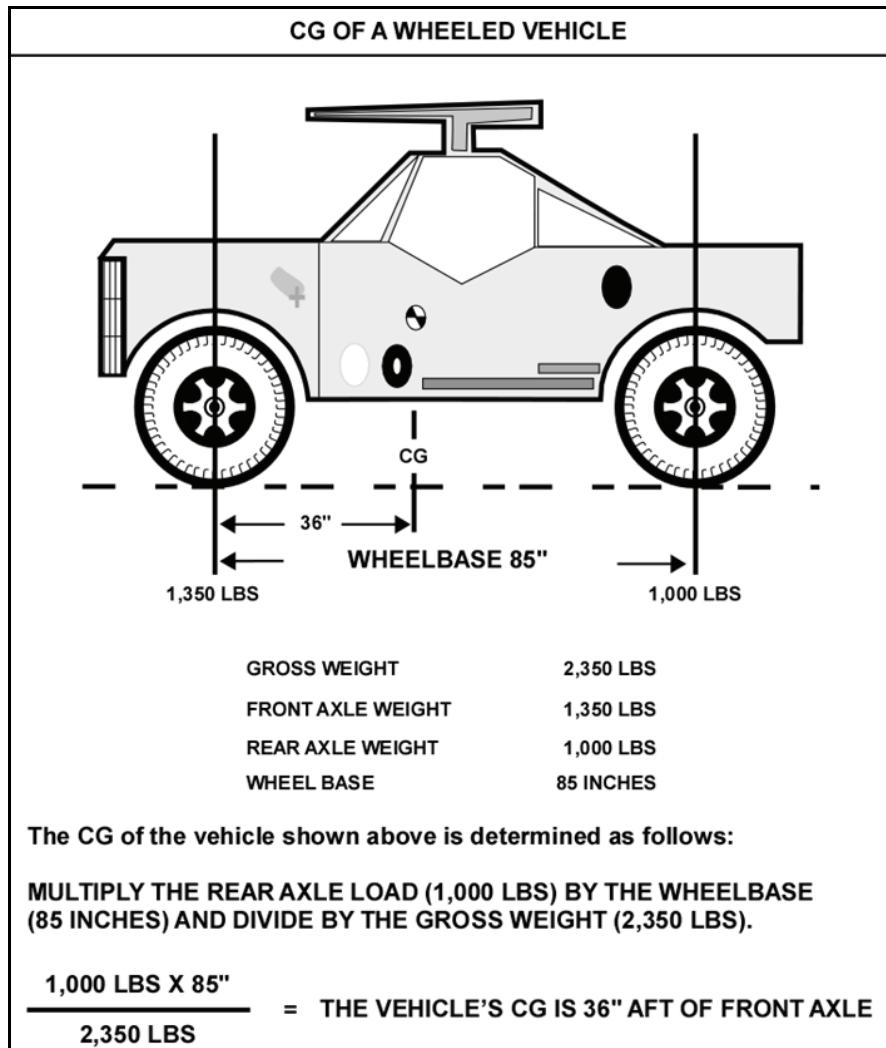
**Figure 2-10. Determining center of gravity of wheeled vehicle**
