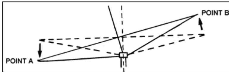
**Figure 1-30. Rotor flapping in response to cyclic input**
