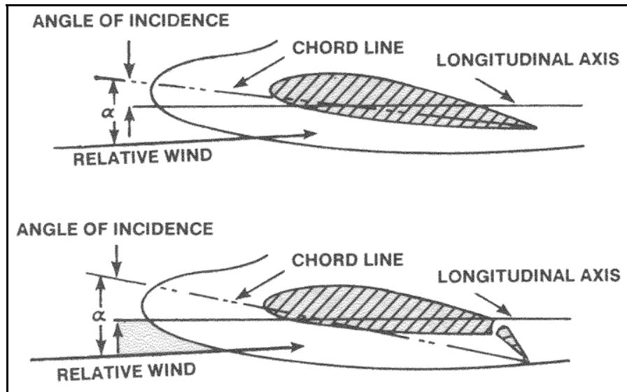
**Figure 7-27. Angle of incidence change with flap deflection**
