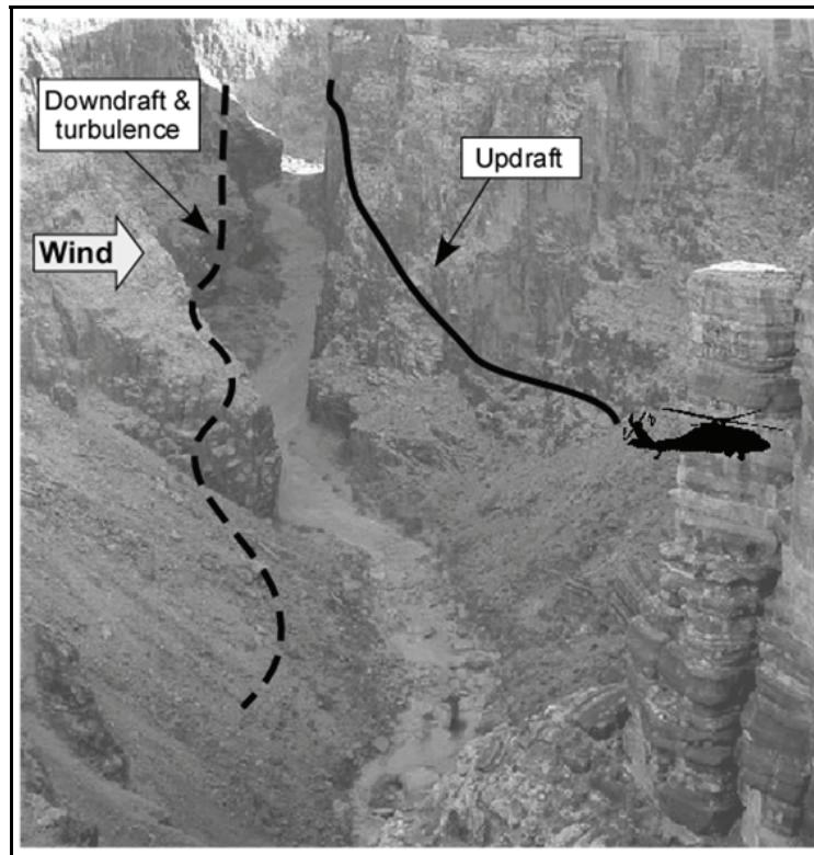
**Figure 3-29. Flight along a valley (terrain flight)**
