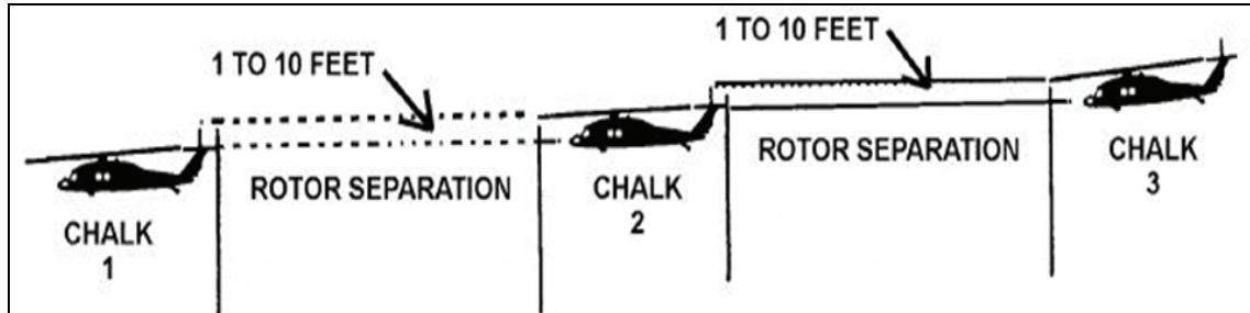
Figure 6-2. Stepped-up vertical separation
