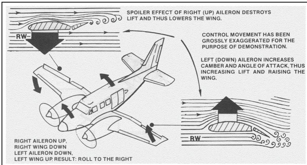
**Figure 7-48. Operation of aileron in a turn**
