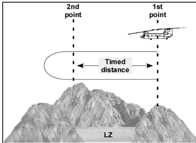
**Figure 3-23. Computing wind direction between two points**
