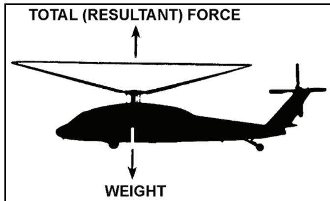
**Figure 1-44. Balanced forces; hovering with no wind**
