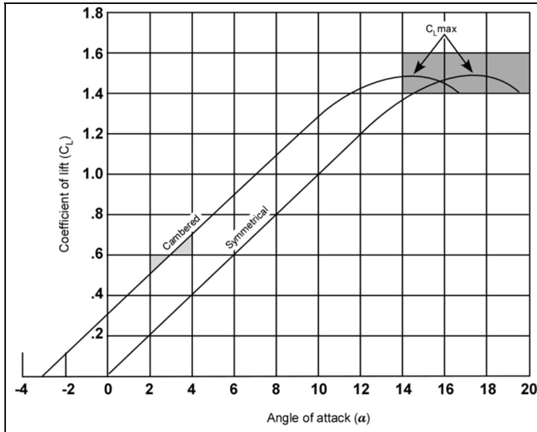
Figure 7-33.  $C_L$  curves for cambered and symmetrical airfoils
