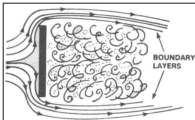
**Figure 7-32. Boundary-layer separation**
