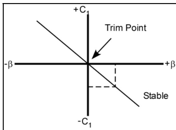
**Figure 7-17. Positive static lateral stability**
