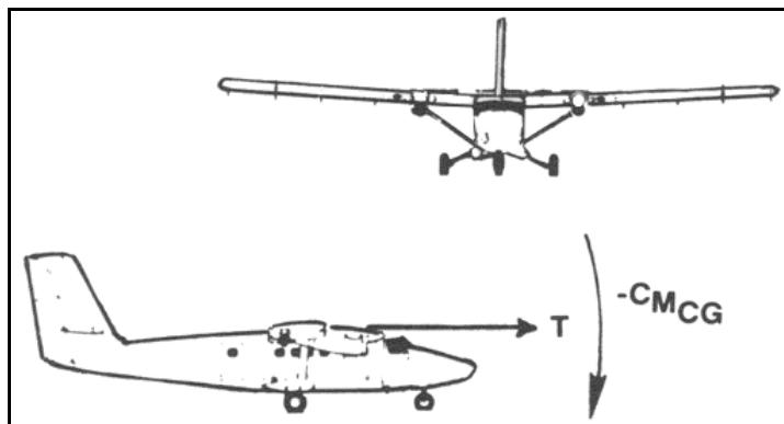
**Figure 7-11. Thrust axis about center of gravity**
