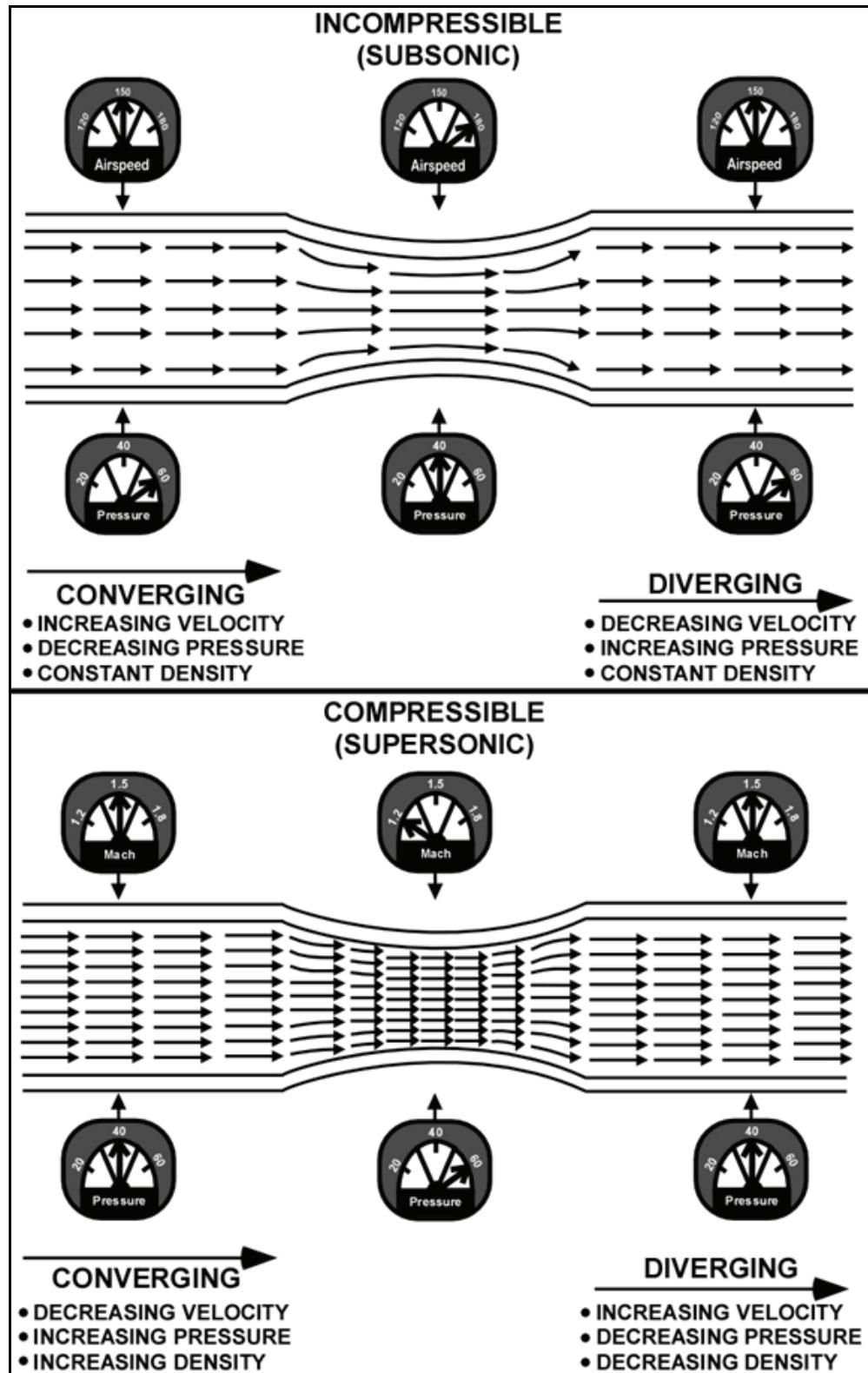
Figure 1-83. Compressible and incompressible flow comparison
