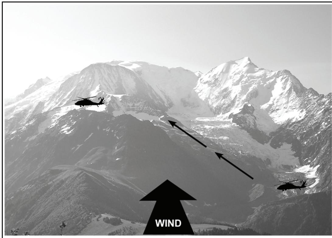
**Figure 3-30. Nap-of-the-earth or contour approach (terrain flight)**
