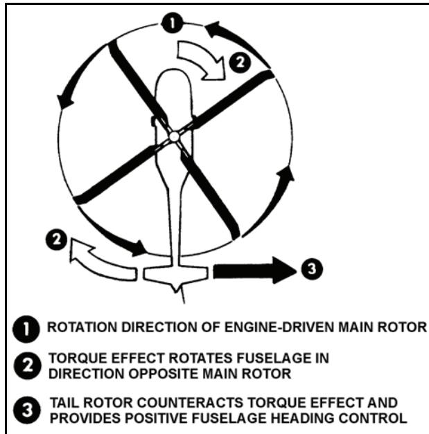
Figure 1-43. Torque reaction
