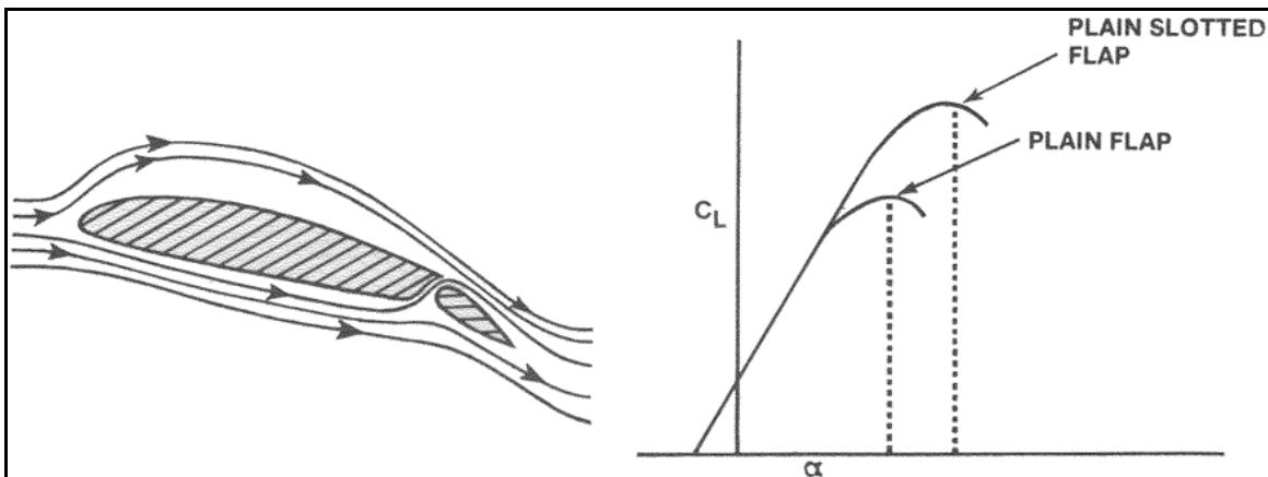
**Figure 7-29.  $C_L$ max increase with slotted flap**
