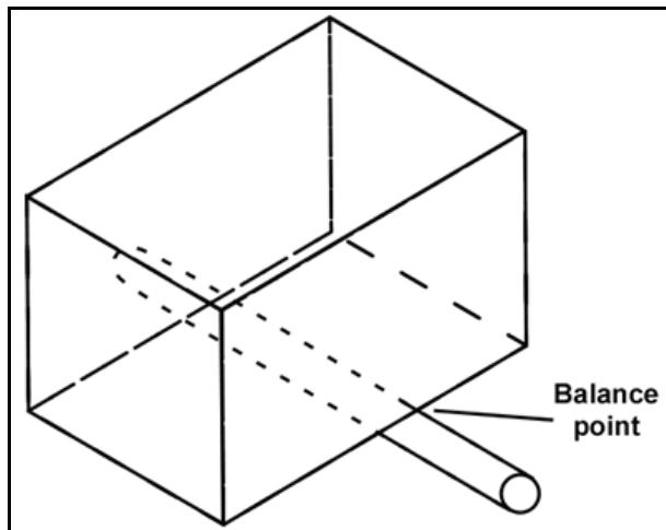
**Figure 2-9. Determining general cargo center of gravity**
