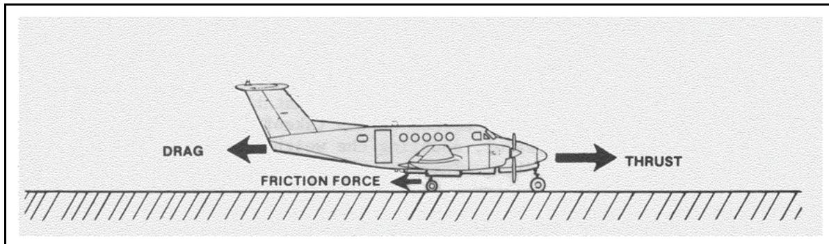
**Figure 7-45. Net accelerating force**
