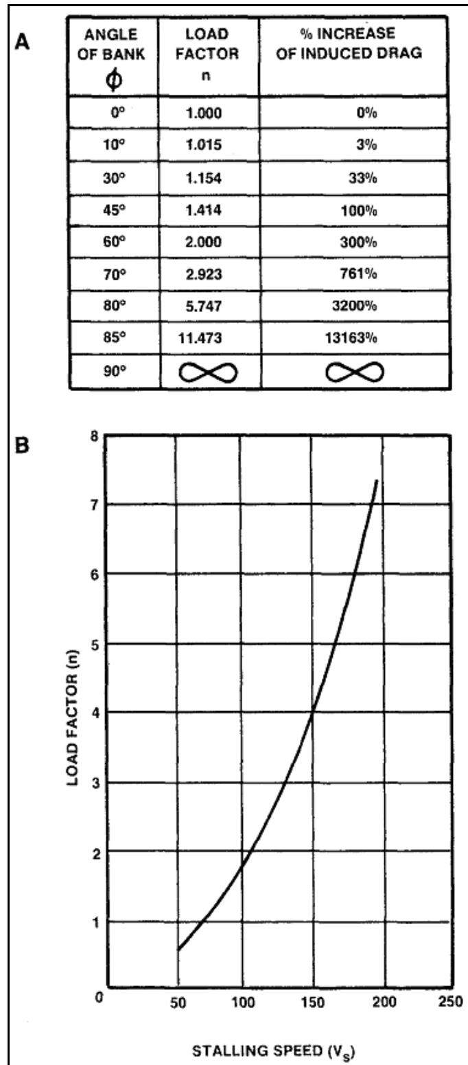
Figure 7-43. Effect of load factor on stalling speed
