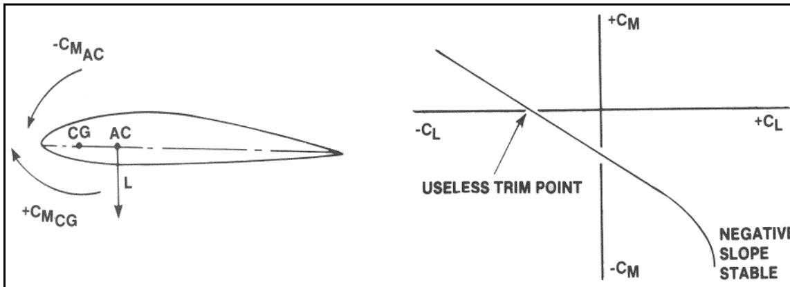
**Figure 7-8. Positive longitudinal stability of a positive-cambered airfoil**
