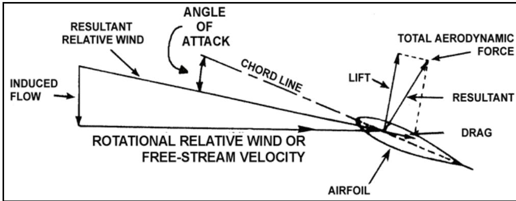
Figure 1-7. Force vectors on an airfoil segment
