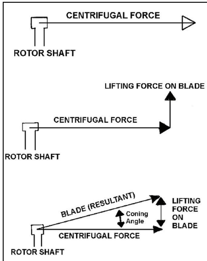
Figure 1-41. Effects of centrifugal force and lift
