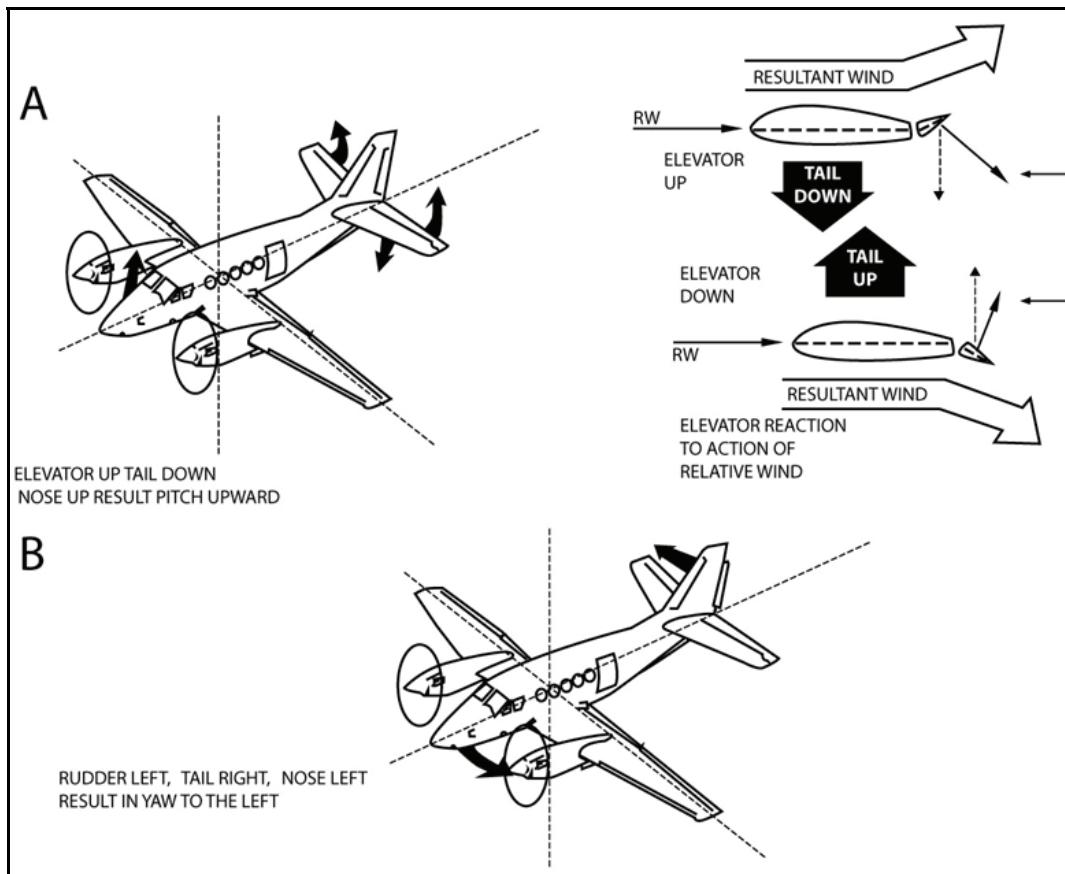
Figure 7-49. Effect of elevator and rudder on moments
