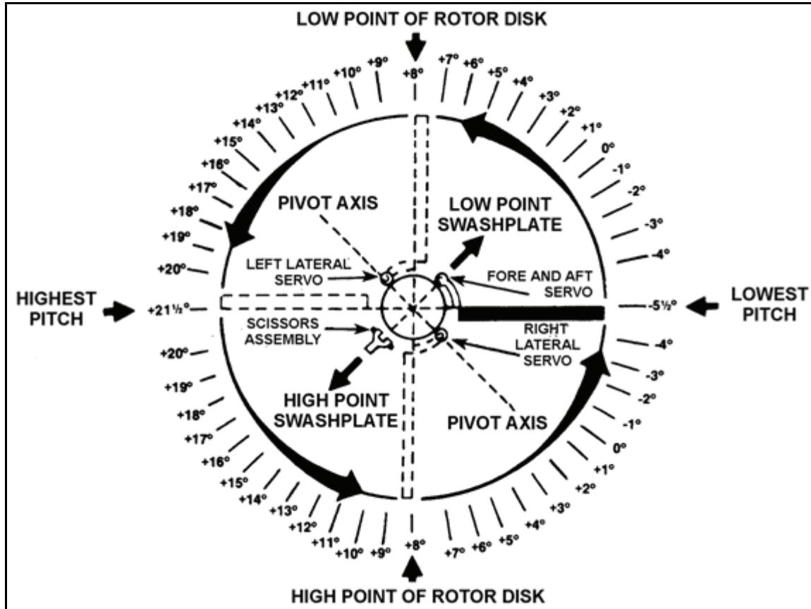
Figure 1-33. Cyclic pitch variation—full forward, low pitch
