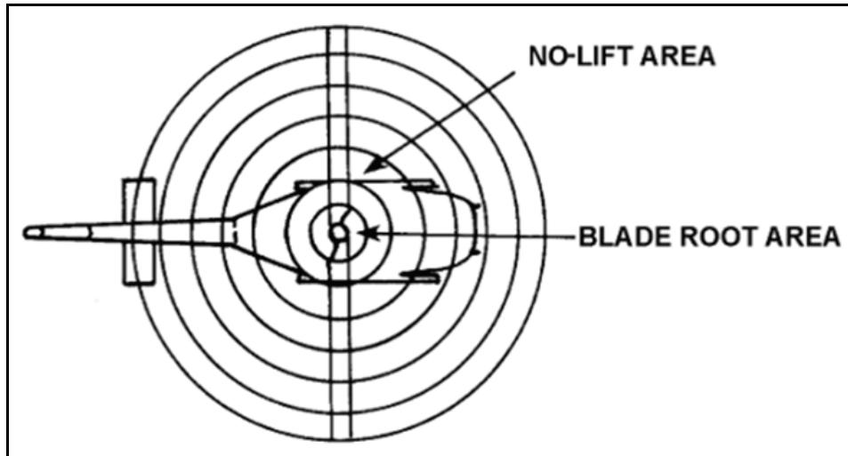
**Figure 1-79. Retreating blade stall (normal hovering lift pattern)**
