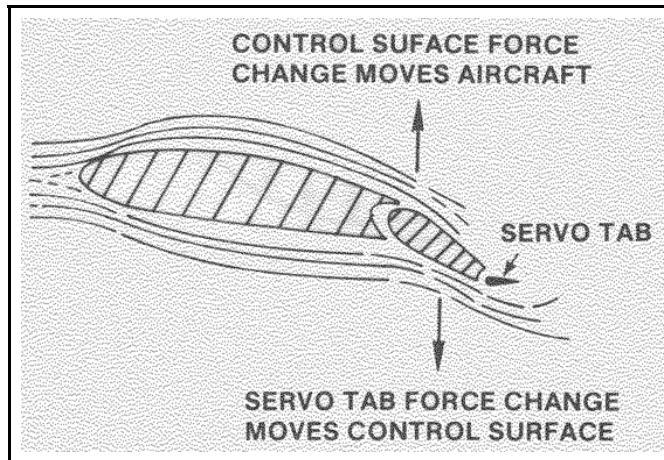
**Figure 7-55. Aerodynamic balancing using a servo tab**
