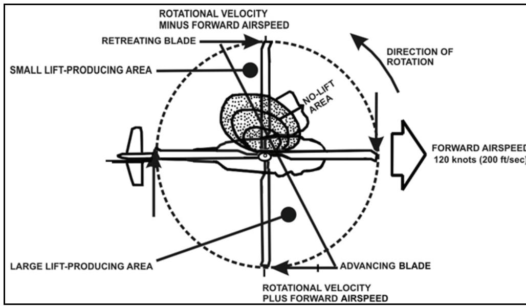
**Figure 1-80. Retreating blade stall (normal cruise lift pattern)**
