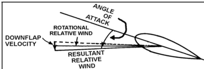
Figure 1-20. Flapping (retreating blade 9 o'clock position)
