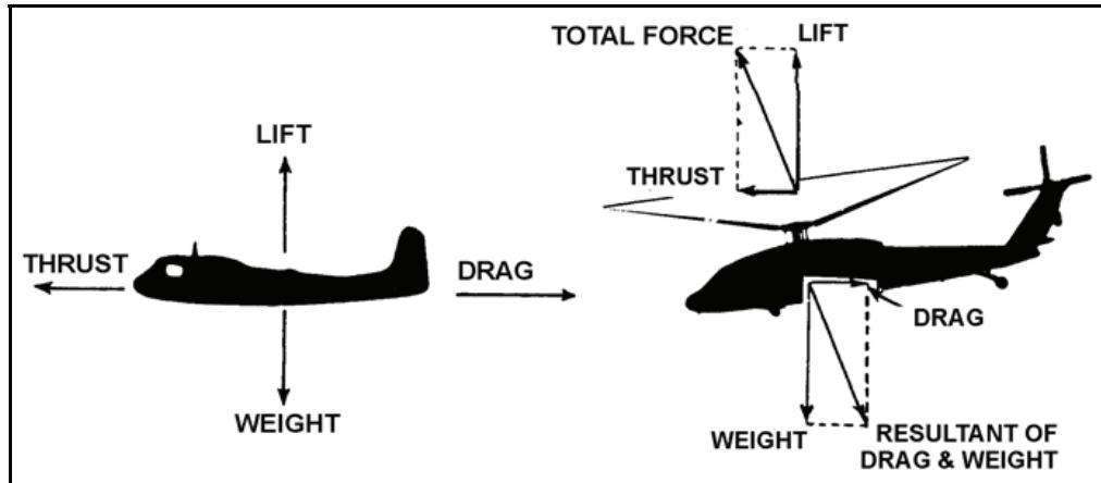
Figure 1-8. Force vectors on aircraft in flight
