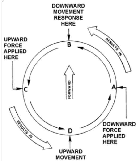
**Figure 1-25. Gyroscopic precession**
