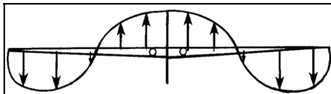
**Figure 1-74. Induced flow velocity before vortex ring state**
