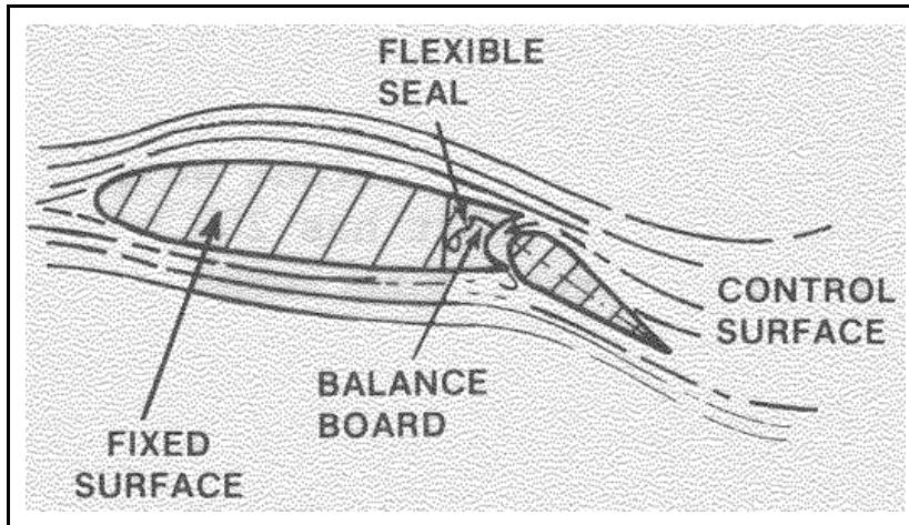
**Figure 7-54. Aerodynamic balancing using a balance board**
