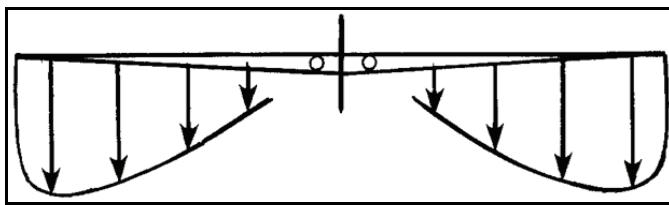
**Figure 1-73. Induced flow velocity during hovering flight**
