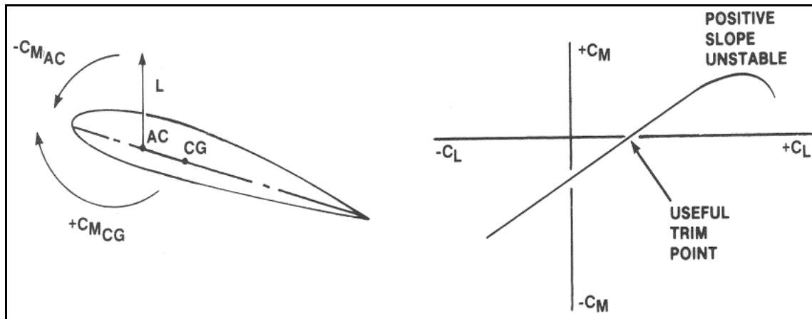
**Figure 7-9. Negative longitudinal stability of a positive-cambered airfoil**
