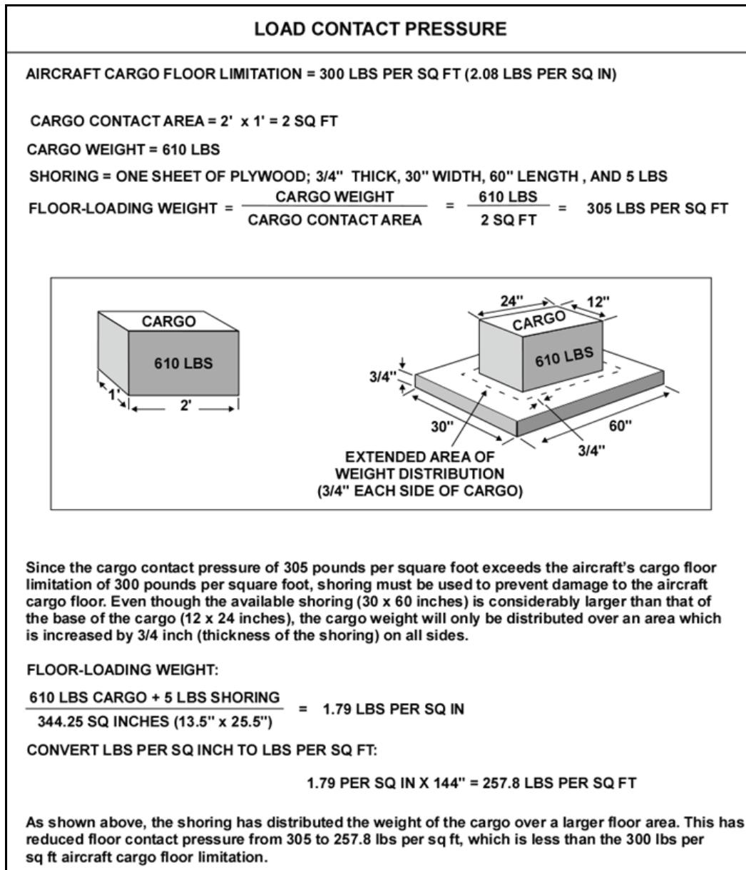
**Figure 2-7. Load contact pressure****Load Pressure Formulas**
