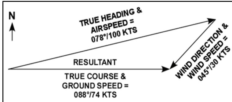
Figure 1-6. Resultant by the triangulation method
