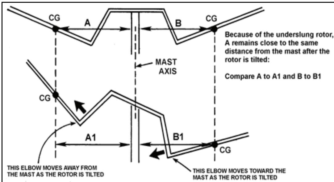
Figure 1-24. Under slung design of semirigid rotor system
