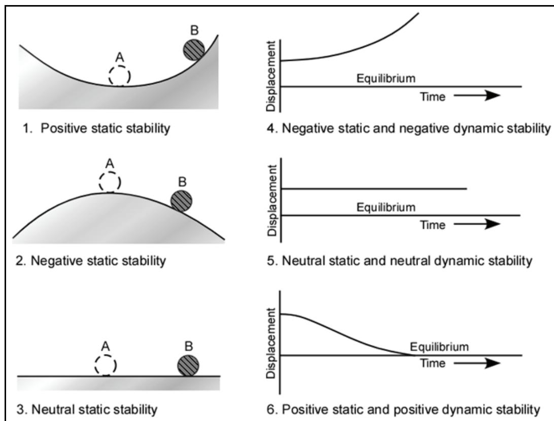
Figure 7-2. Nonoscillatory motion
