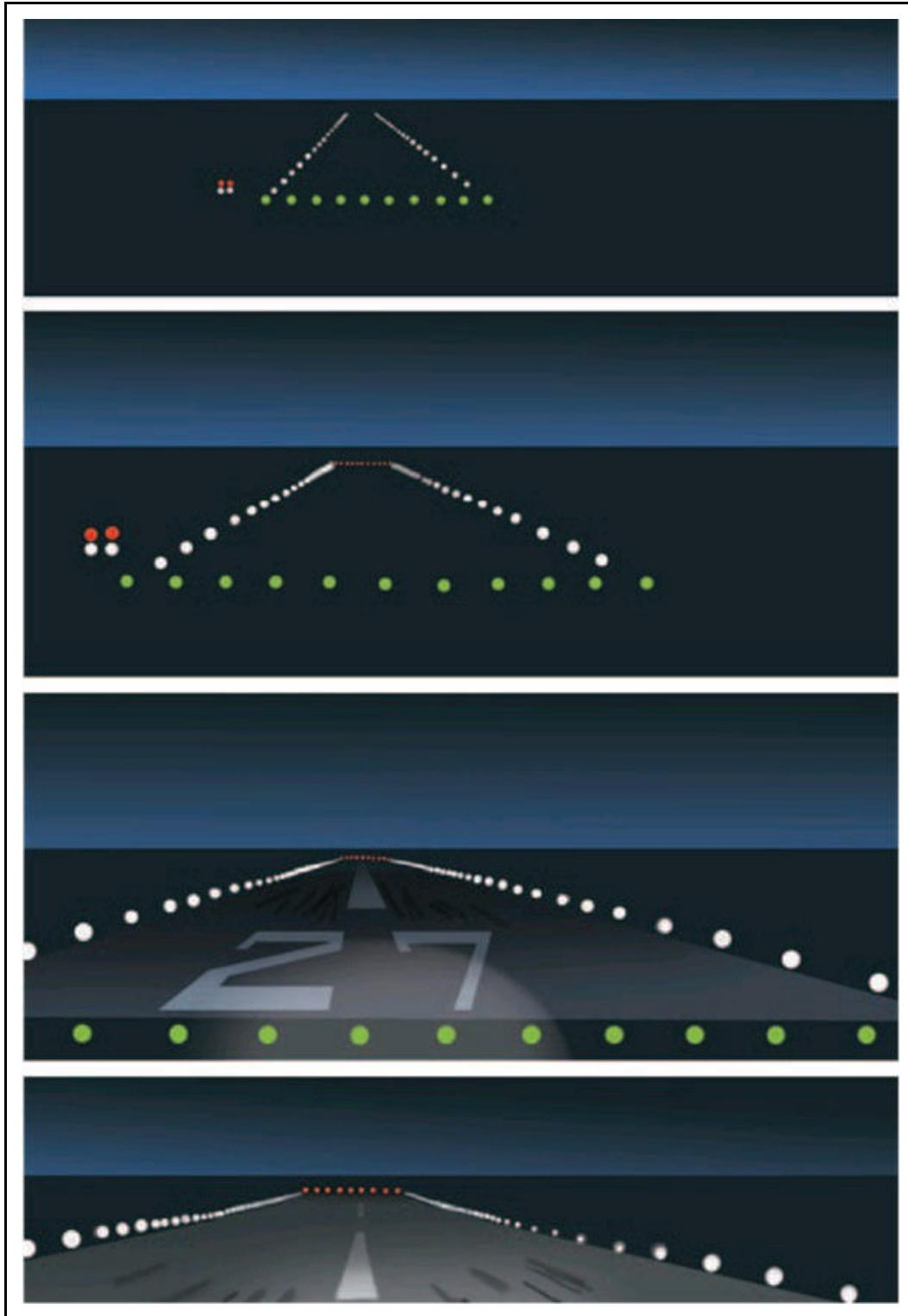
**Figure 9-4. Roundout (when tire marks are visible)**
