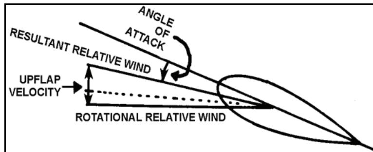
Figure 1-54. Flapping (advancing blade, 3-o'clock position)
