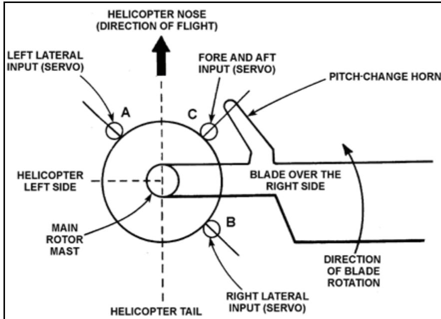
**Figure 1-32. Input servo and pitch-change horn offset**
