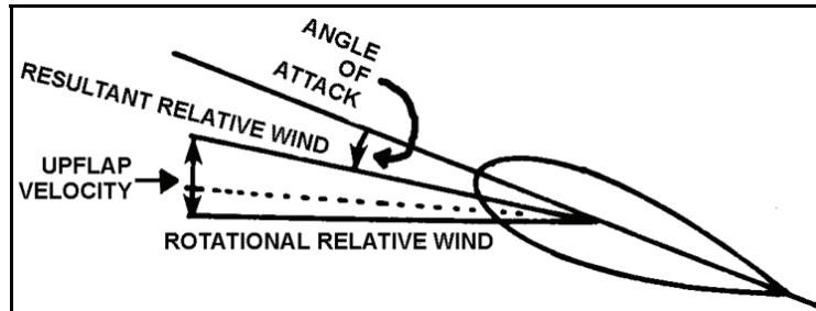
Figure 1-19. Flapping (advancing blade 3 o'clock position)
