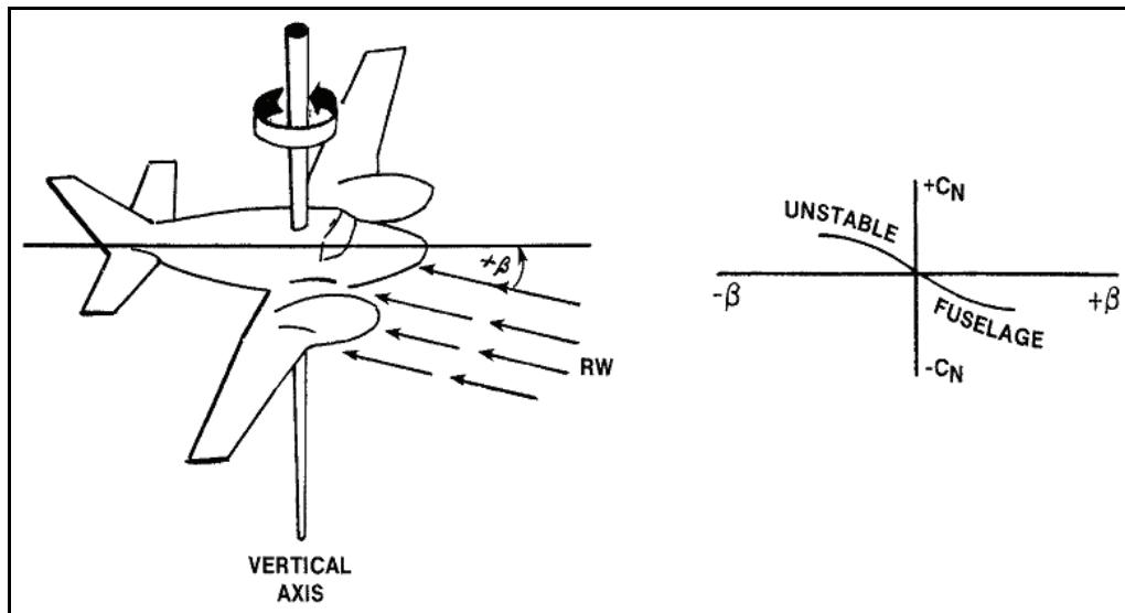
**Figure 7-13. Directional stability ( $\beta$  versus  $C_N$ )**
