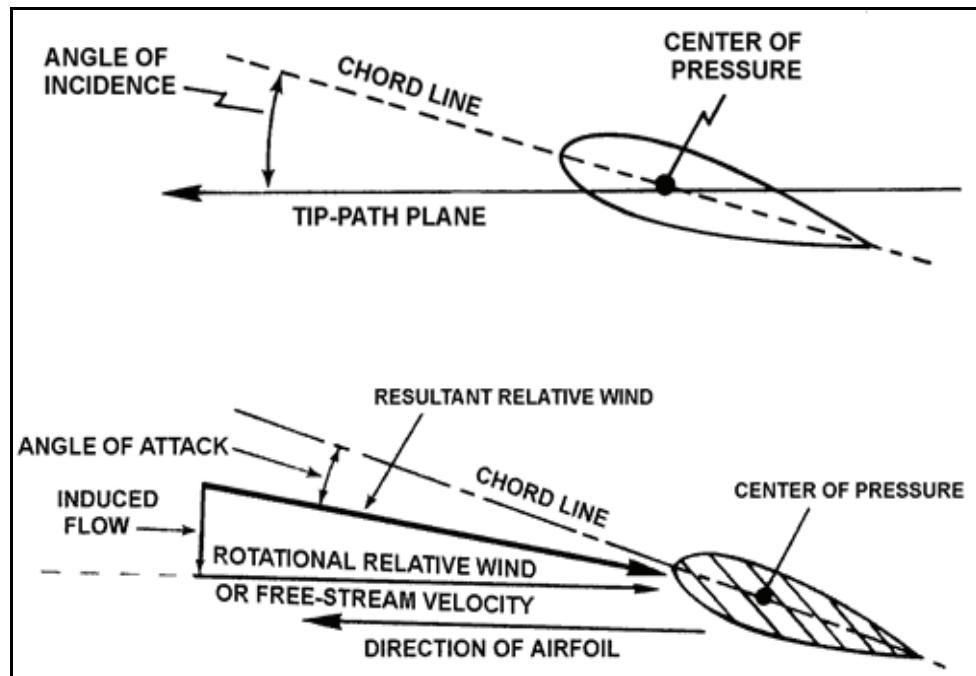
Figure 1-15. Angle of incidence and angle of attack
