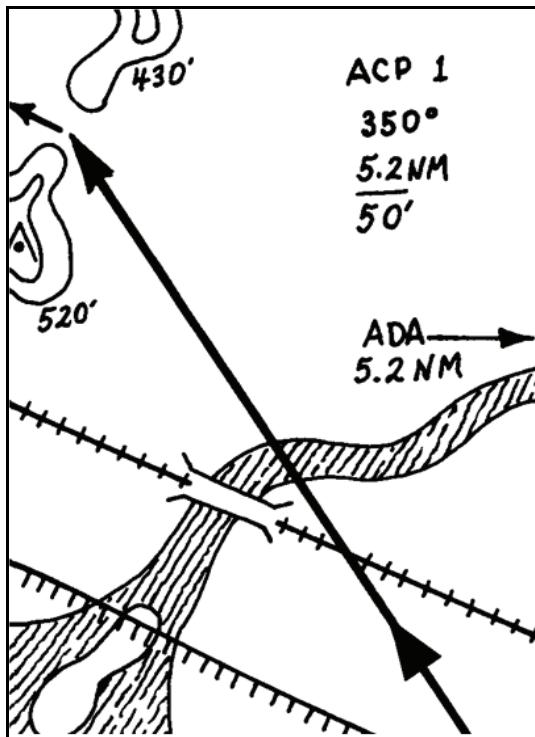
**Figure 5-4. Example of an en route card**
