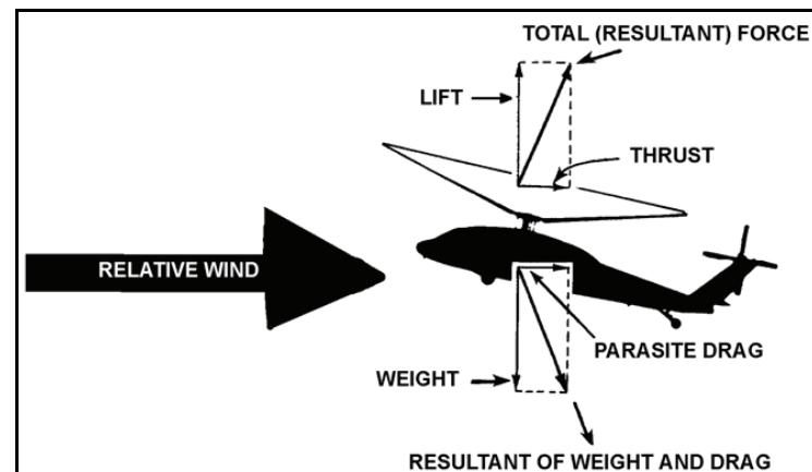
**Figure 1-47. Unbalanced forces causing deceleration**
