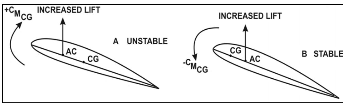
**Figure 7-6. Wing contribution to longitudinal stability**
