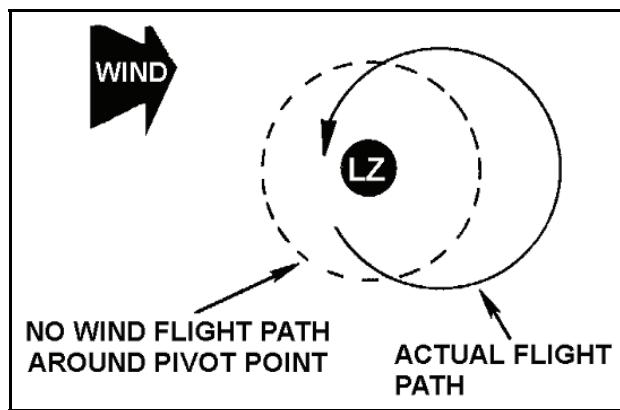
**Figure 3-24. Computing wind direction using the circle maneuver**
