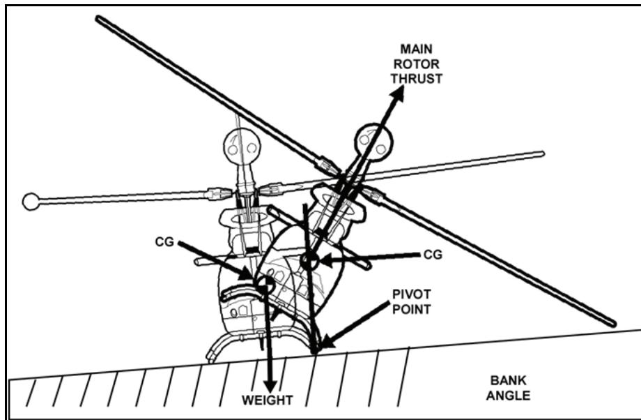
Figure 1-78. Upslope rolling motion
